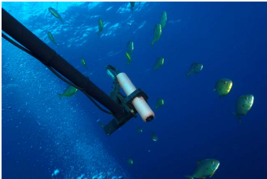
Fig 1. HyperOCR at 9 m protected with copper tape for avoiding bio-fouling.
